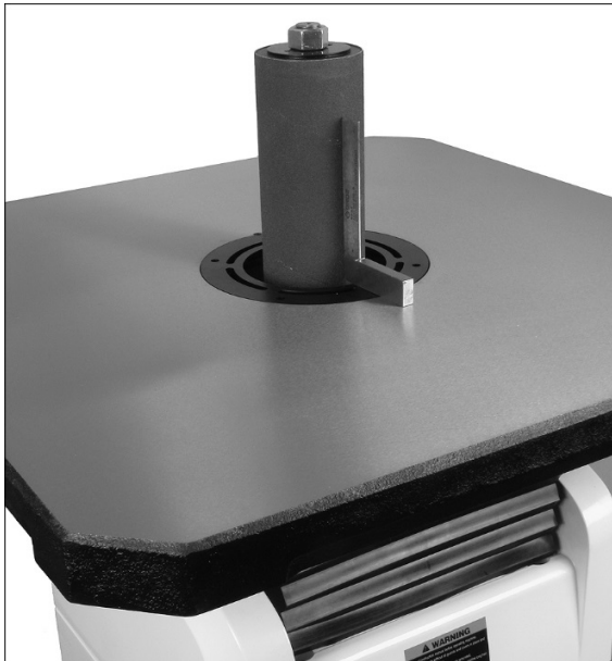
Figure 13: setting tilt stop
